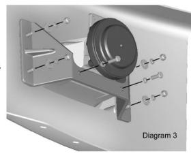
Diagram 1 (Tilt and insert speaker assembly)
