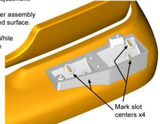
5) Insert the 3/8-16 x 1.25" carriage head bolts (item 6) into the four cast slots on the wedge bracket. To hole these bolts in place, push the 5/16" nylon push retainer (item 4) onto the threads of each 3/8" bolt, all the way up the length of the threads. See diagram at right.
